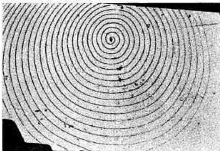
Figure 1: Growth spiral on a carborundum face. Crystallographic Laboratory, Geological Institute, University of Ghent.
