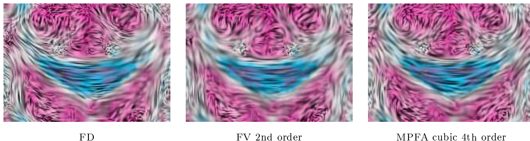
Figure 3.1: Artificial diffusion in different numerical schemes. Crops from colorized MR-DTI visualizations based on real data, transverse plane slice.
