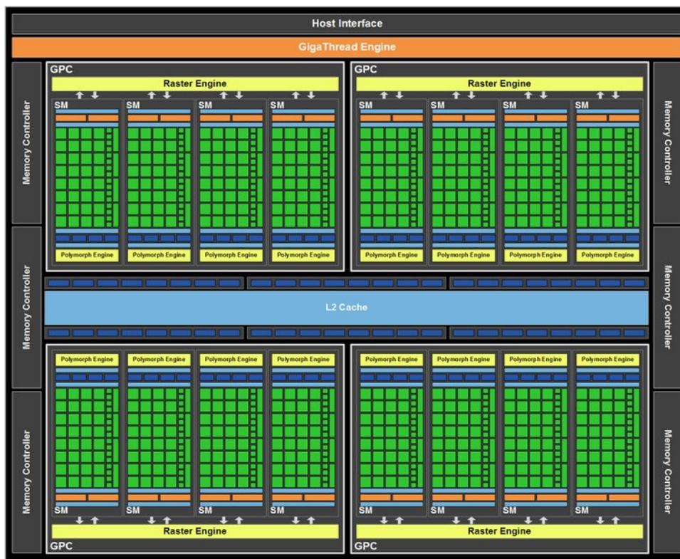
Figure 3: Die schema of Fermi microarchitecture consisting of 16 streaming multiprocessors (SM) coalesced into four graphics processing clusters (GPC)
