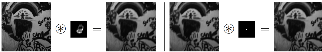
Figure 1: This figure illustrates difference between ground-truth and no-blur solution. On the left side, there is a convolution of ground-truth solution, on the right side, there is a convolution of the no-blur solution. The image and PSF are taken from the Levin dataset.
